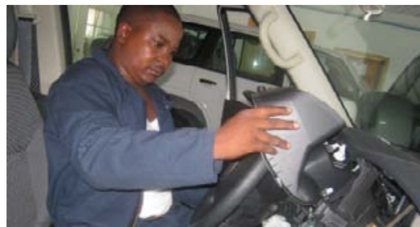
John Nyaga fitting the dismantled parts after installing the car log gadget
